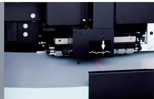
AMS suction cover feed with score indicator
